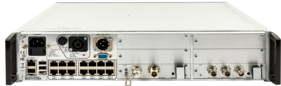
The LD6 Integrated Mobile Unit data ports.
